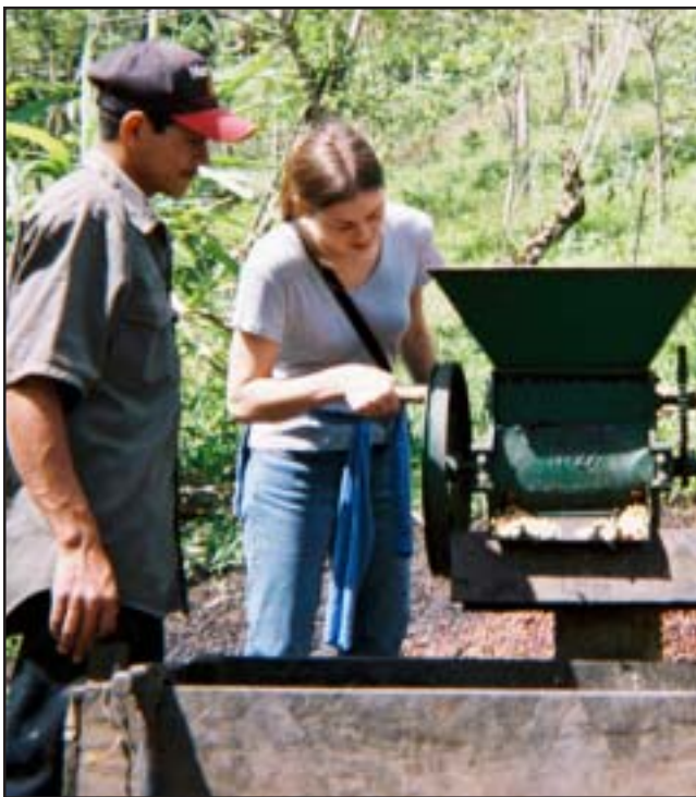
AFTER PICKING A BASKET OF COFFEE CHERRIES, Julia runs them through a depulping machine. The beans are then washed and dried and the pulp is composted and used as organic fertilizer.
